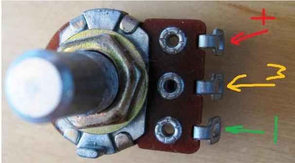
To toggle "pot mode" on and off, hold down the up, down and left keys for 10 seconds. When the command is accepted, the light will flash in an alternating pattern of 0101 and 1010. When in pot mode, the brightness of the pulse LED is controlled by the potentiometer position. This is a good check to make sure that the pot is hooked up correctly, and serves as a visual indicator that the board is currently set in pot mode.
